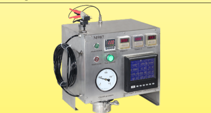
Test equipment for measuring repeatedly and constantly the maximum length of the air switch connecting tubes according to the volume of the push button and the pressure it develops (Ultimheat Laboratory)
